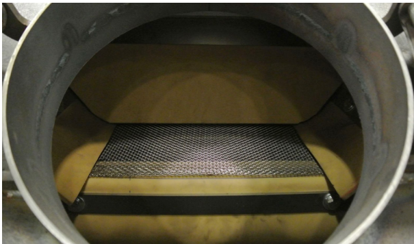
Belt screen with vibrator assist mounted underneath for minimal surface area interruption. ALL PHOTOS: © ATLANTIC DESIGN, INC.
