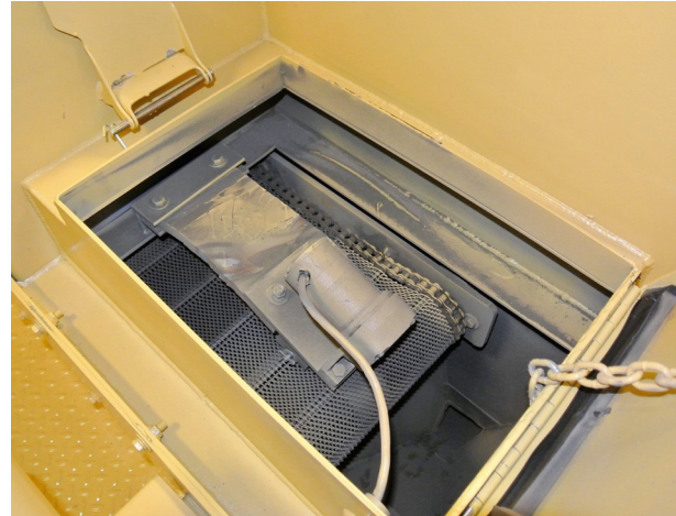
Belt screen with vibrator assist mounted on top.
